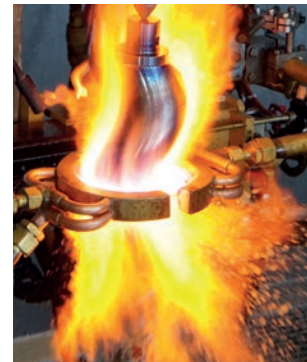
Rotor at flame-hardening process
