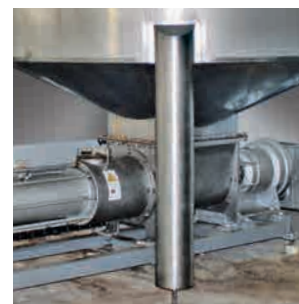
Feed process in a KL100RL120-8 V4A progressing cavity pump
